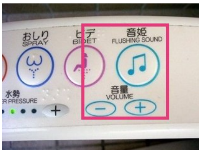
Figure 4. Otohime (with FLUSHING SOUND in English) with volume control on the control panel of a washlet (Start and stop the flushing sound by pressing the FLUSHING SOUND button; control the volume by pressing – or + of VOLUME)
