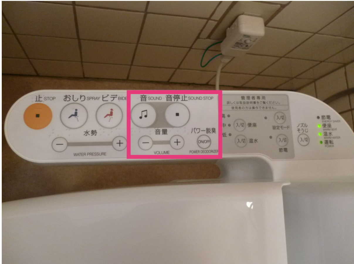
Figure 3. Otohime (with SOUND and SOUND STOP in English) with volume control on the control panel of a washlet (Start the flushing sound by pressing the SOUND button and stop it by pressing the SOUND STOP; control the volume of the flushing sound by pressing – or + of VOLUME)
