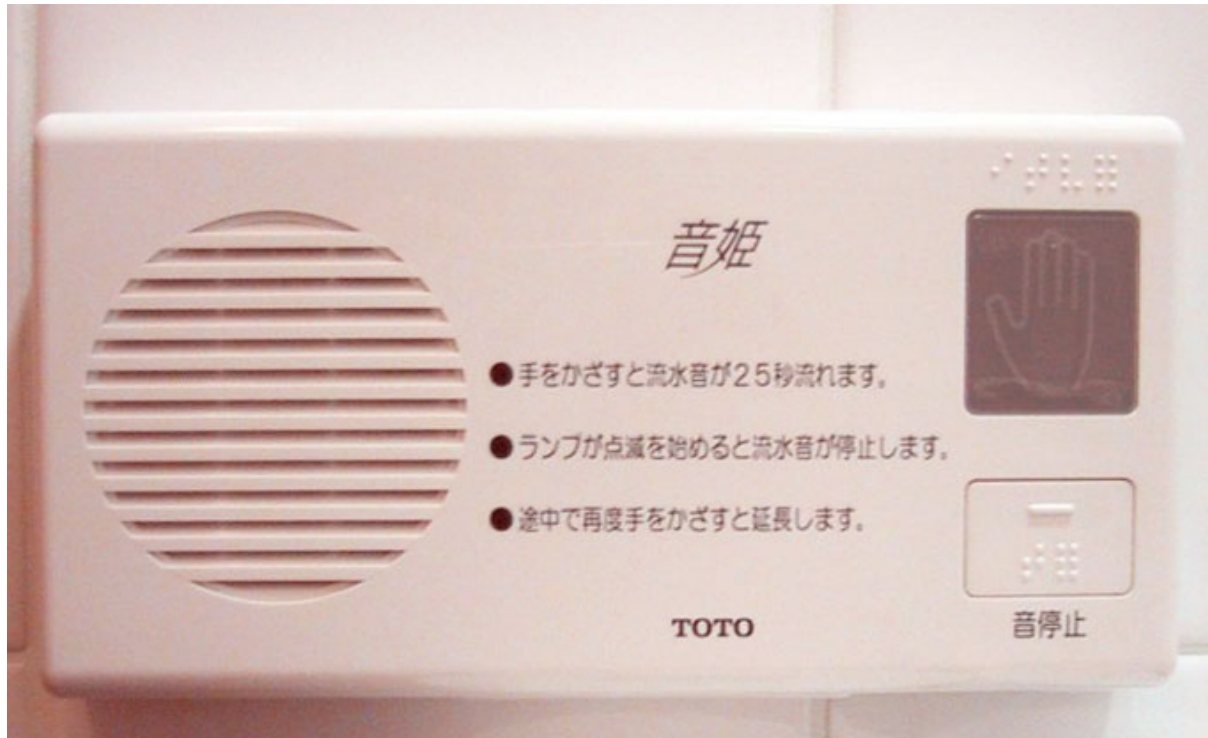
Figure 1. A stand-alone Otohime (Japanese only) on the wall of a toilet booth (by waving hand to the upper right corner, the flushing sound will be played for 25 seconds; lengthen the sound by waving hand again; stop the sound halfway by pressing the Stop button at the lower right corner)
